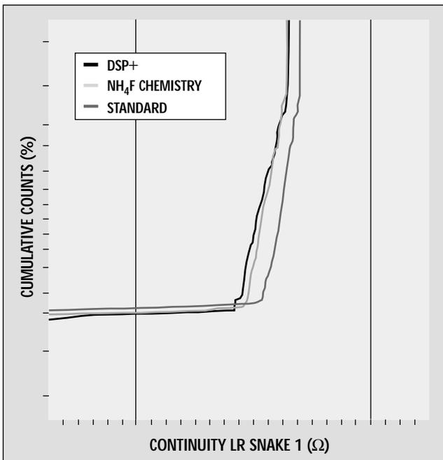
**Figure 8: Electrical tests of devices presented in Figure 7. Snake continuity measurements demonstrate that the use of the DSP mixture produces structures with lower resistivity than the process of record.**
