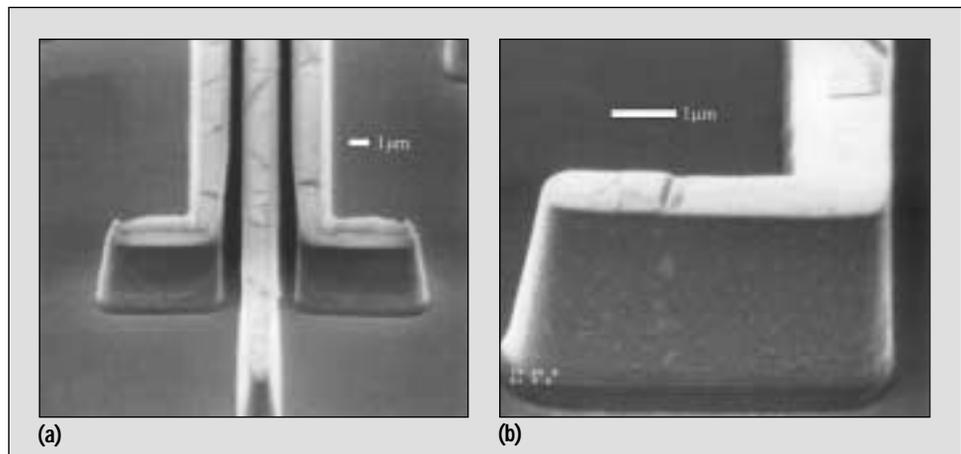
**Figure 4: SEM images of a metal 6 stack (a) before and (b) after exposure to the DSP mixture.**
