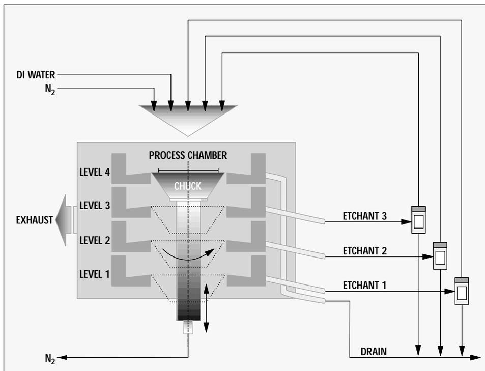
**Figure 2: Schematic drawing of the spin-processor chamber.**
