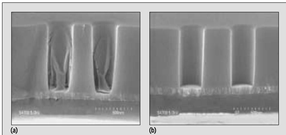
**Figure 6: SEM images of a contact/via 6 structure cleaned with the DSP mixture for 90 seconds.**
