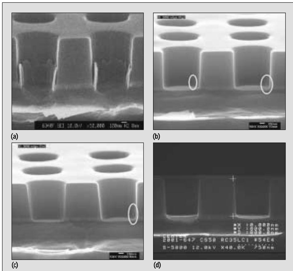
**Figure 5: SEM images of contact/via 6 structures: (a) before cleaning; (b, c, and d) different structures processed under differing conditions after the initiation of residue cleaning.**
